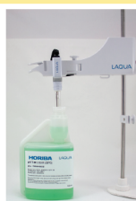
Step 3: Insert the electrode into the calibration chamber of the standard solution bottle.
