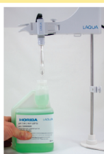
Step 2: Gently squeeze the bottle to fill the calibration chamber with standard solution.
